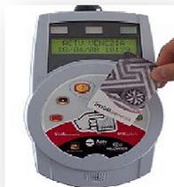
*Figura 7 - Contactless smartcard*
