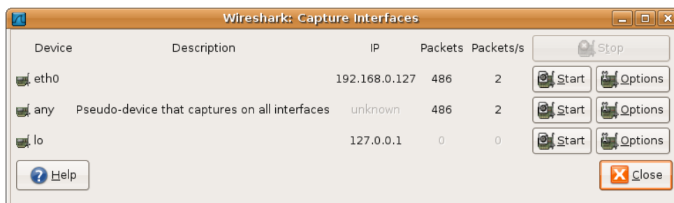
Figure 4.2. The "Capture Interfaces" dialog box on Unix/Linux
